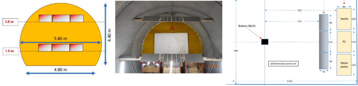
Fig. 4. Position of collector plates, textile, PC, and corrosion metal plates, test site A, experiment 1.
