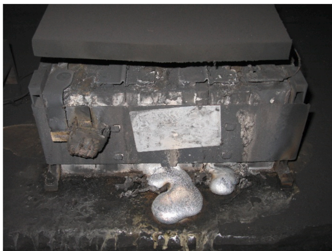
Fig. 17. Molten aluminum leaked from the battery.
